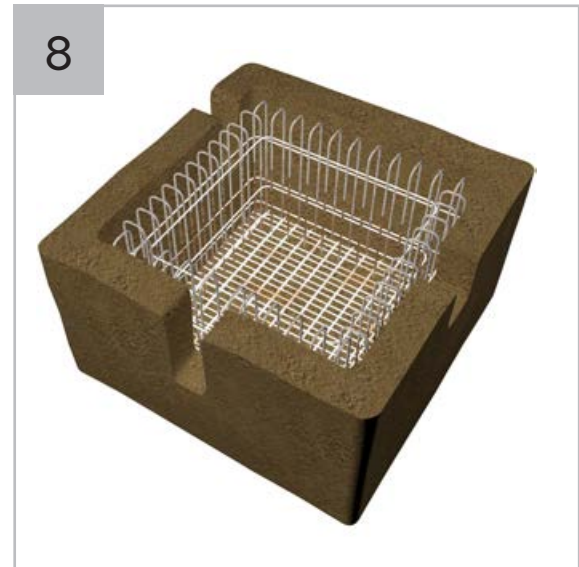
Install re-bar as per structural engineer's details.
