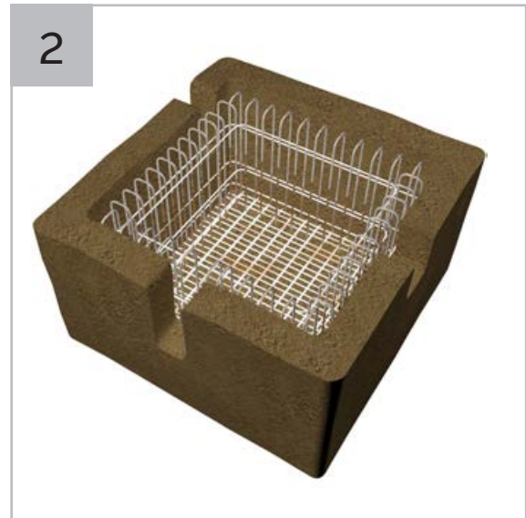
Install re-bar as per structural engineer's details.
