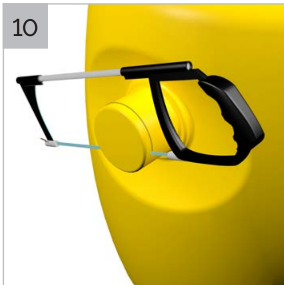
10 Saw off socket ends, where inlet pipes are to be connected.
