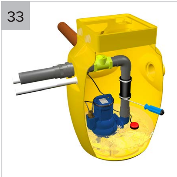
Tighten the jubilee clips to seal the rubber drain coupling to the pipe.
