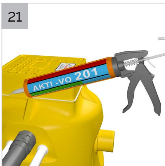
Once chamber has been filled with water, apply Delta AKTI-VO 201 (swellable mastic) to the entire external lip locator of chamber.
