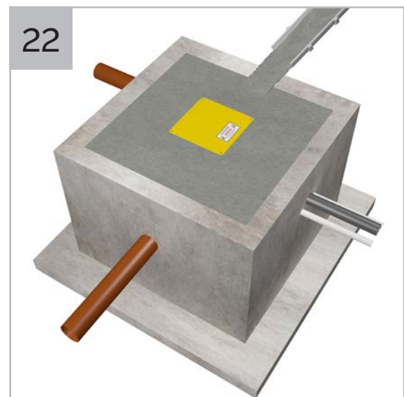
Fill void between RC box and chamber with concrete (we recommend use of C35 grade/PAV2 as a minimum) or as per the structural engineer's details.
