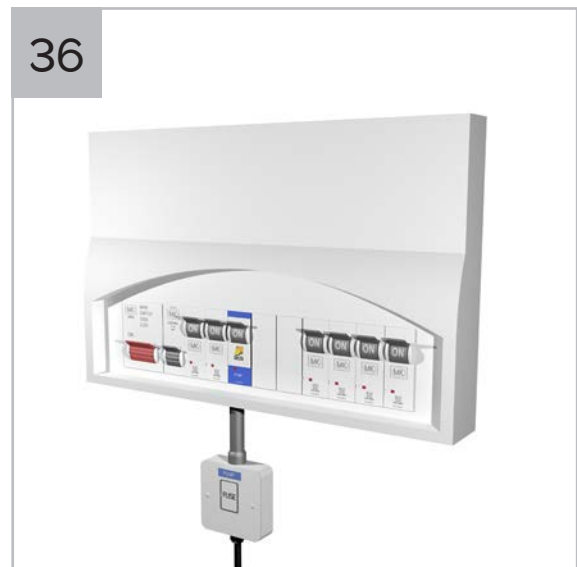
Isolate main supply and connect the pump to a separate non-switched fused spur. When installing a Delta HLA, follow the wiring diagram on page 18.
